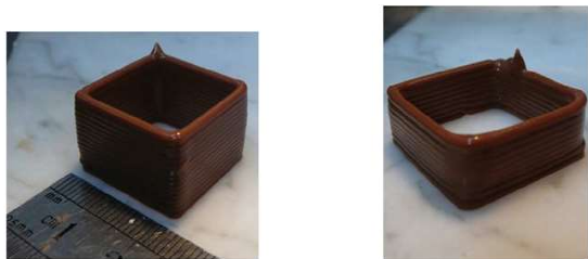
Figure 4. The chocolate square with good layer-by-layer bond and geometry accuracy. Figure 5. The chocolate square with poor geometrical accuracy.
